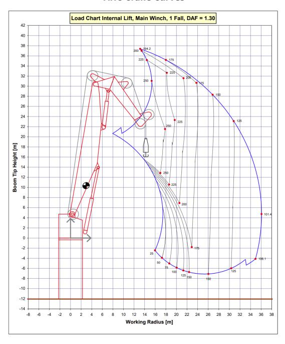
Max lift capacity: 250 t/ 18 m Max outreach: 100 t/ 36 m
